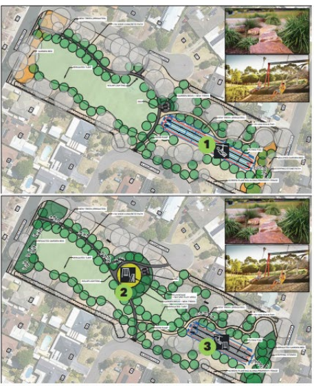
Proposed concept plans show examples of option 1 large flying fox, option 2 basket swing and small slide, option 3 standard flying fox and basket swing. Please note option 4 is no play equipment with additional greening across the reserve.
